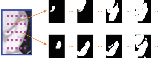
Fig. 3. Seed hypotheses. The small magenta squares represent different foreground seeds placed in rectangular grid. The bold blue lines at image borders represent background seeds. We also present the segmentation proposals for two different foreground seed hypotheses. In each set of proposals, \lambda increases from left to right. (Color figure online)
