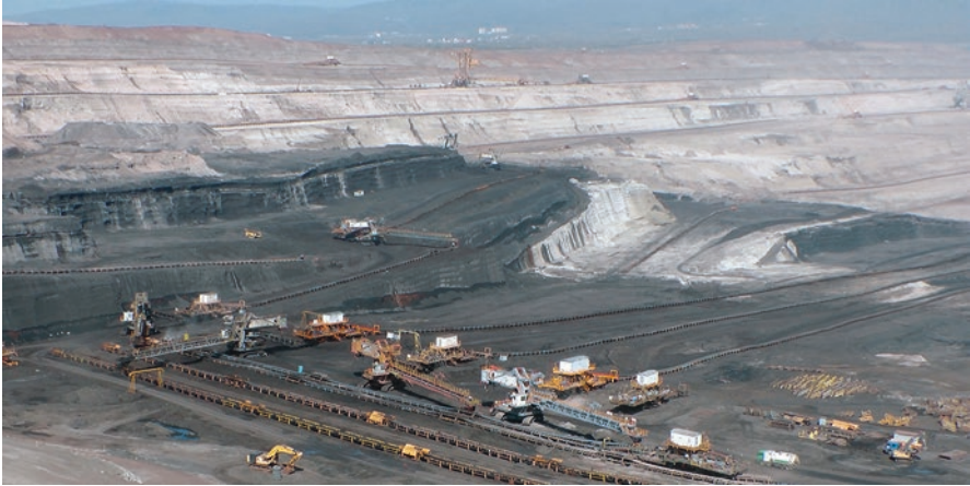
Fig. 4.1 Coal surface mine with mining equipment such as excavators and conveyors
