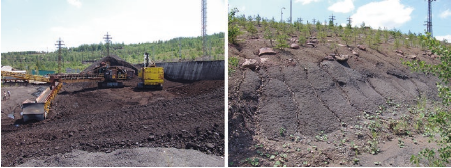
Fig. 4.23 Mapping the surface coal mine with 3D laser scanner HDS3000 (on the left side) and GPS (on the right side)
