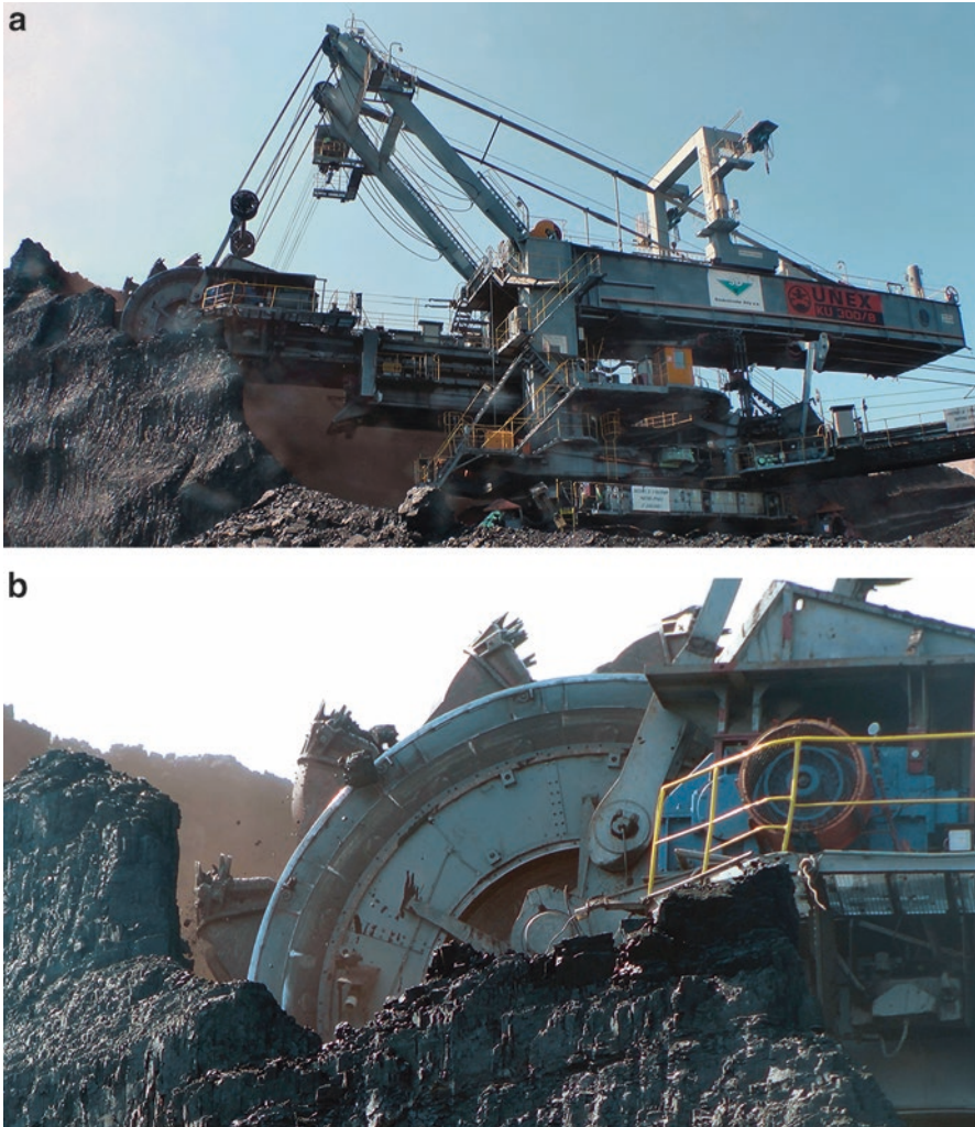
Fig. 4.2 (a) Coal extraction in a surface mine with an excavator. (b) The extraction of coal by an excavator in a detail view
