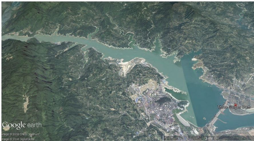
Fig. 5.15 Three Gorges Dam: China, 30°49'15"N 111°00'08"E, capacity 22,500 MW (creates Three Gorges Reservoir, total capacity 39.3 km 3 , catchment area 1000,000 km 2 , surface area 1084 km 2 , max. length 600 km, normal elevation 175 m). Source: Google Earth, 2016
