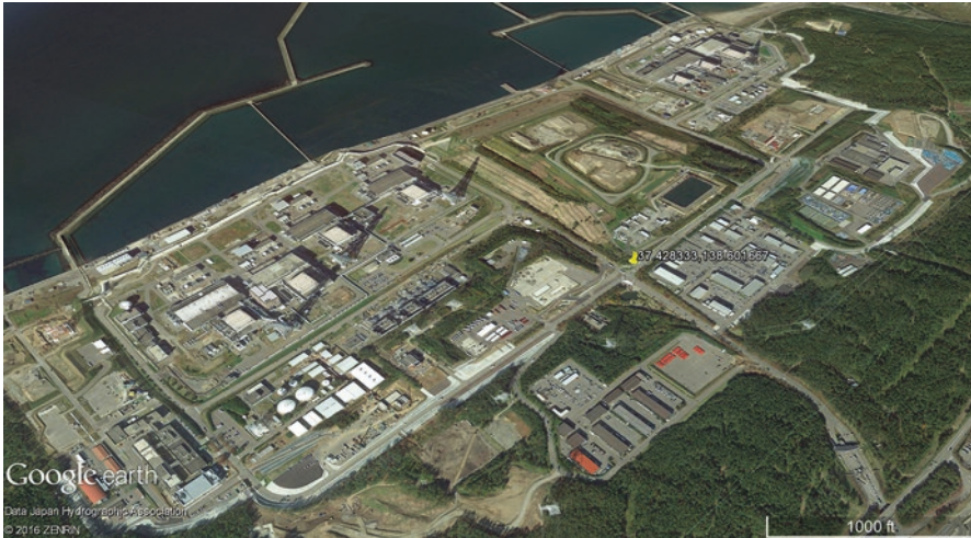
Fig. 9.2 Kashiwazaki-Kariwa Nuclear Power Plant in Japan with the nameplate capacity 7965 MW (7 operational reactors: 5 × BWR 1067 MW; 2 × ABWR 1315 MW). Source: Google Earth, 2016
