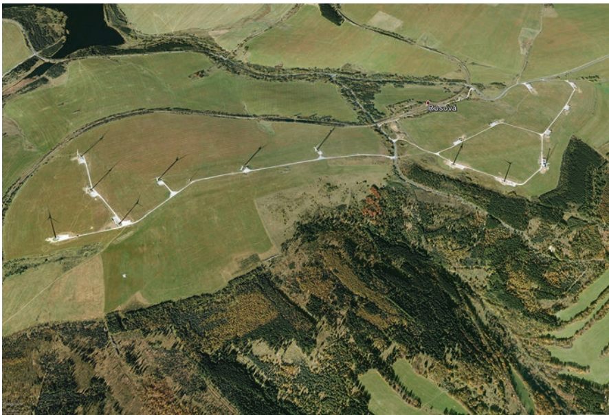
Fig. 6.21 A part of the regional wind farm (42 MW, 21 turbines, estimated production 100 GWh). Google Earth, 2016
