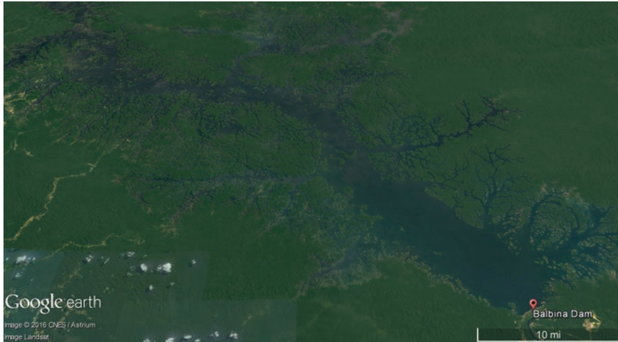
Fig. 5.18 Balbina Dam: Brazil, 01°55'02"S 59°28'25"W, capacity 250 MW (creates Balbina Reservoir, total capacity 17.54 km 3 , catchment area 16,502 km 2 , surface area 2360 km 2 , max. water depth 30 m). Source: Google Earth, 2016
