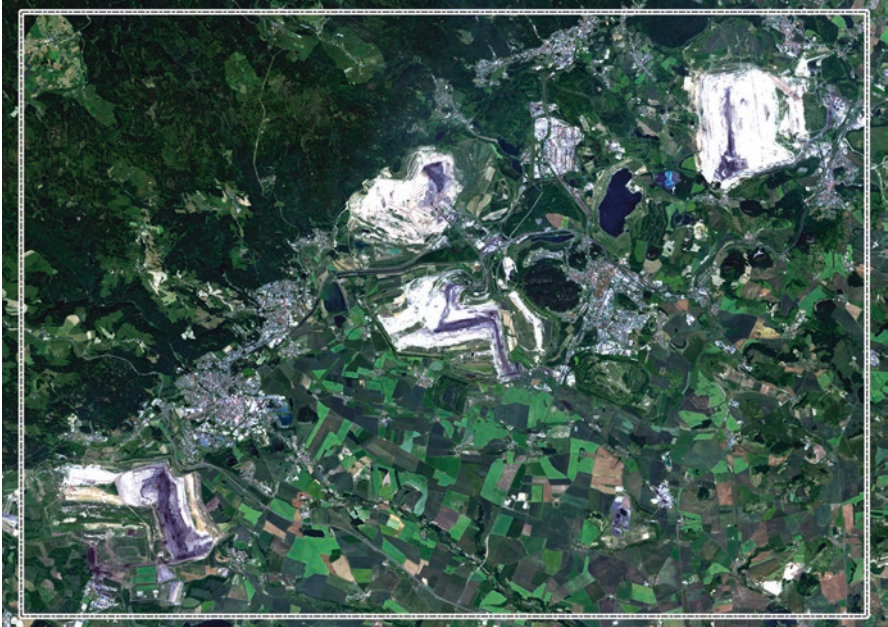
Fig. 4.27 Landsat 8 image (June 24, 2016) in visible spectrum (OLI band: 4, 3, 2), mines are indicated by light sites
