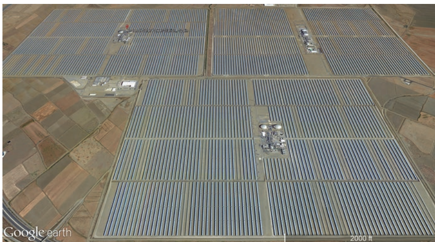
Fig. 10.6 The Andasol solar power station (150 MW), Europe's first commercial plant to use parabolic troughs, located near Guadix in Andalusia, Spain. Source: Google Earth, 2016
