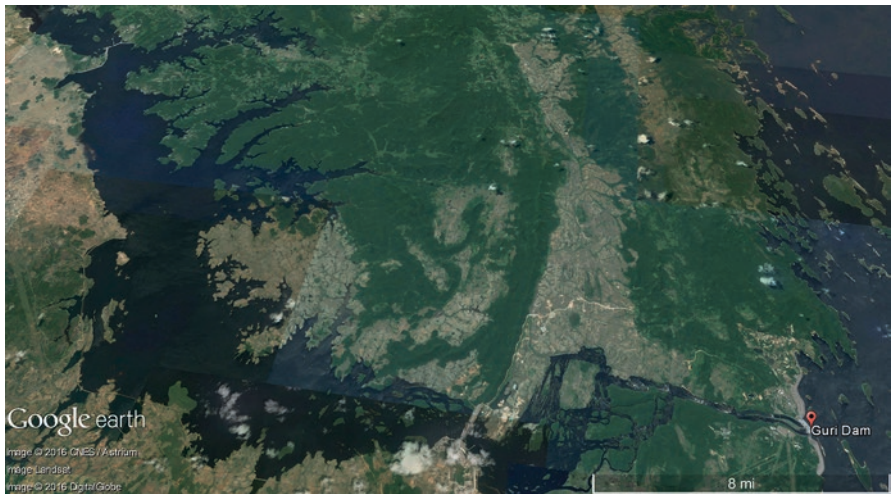
Fig. 5.17 Guri Dam: Venezuela, 07^{\circ}45'59''\text{N} 62^{\circ}59'57''\text{W} , 10,200 MW (creates Guri Reservoir, total capacity 135 \text{ km}^3 , surface area 4250 \text{ km}^2 ). Source: Google Earth, 2016
