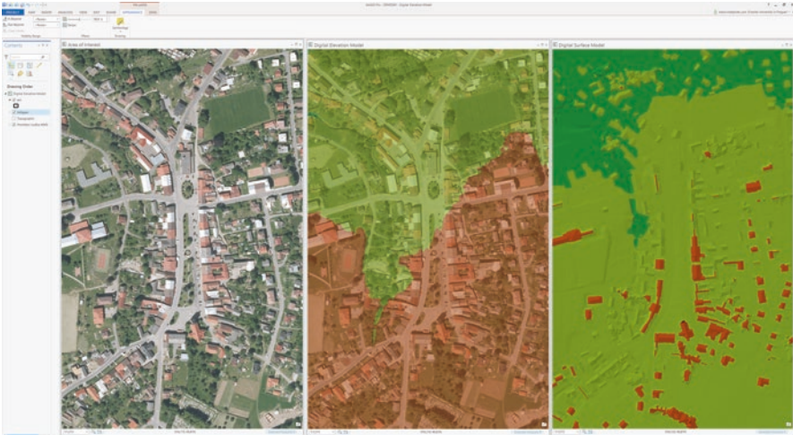
Fig. 2.10 Raster algebra applied on building of the digital surface model (DSM) in ArcGIS Pro (ortofoto of a residential area on the left side, DEM in the middle part, and DSM on the right side; the DEM and the DSM are displayed in different elevation intervals represented by color classes in order to recognize surface objects properly)
