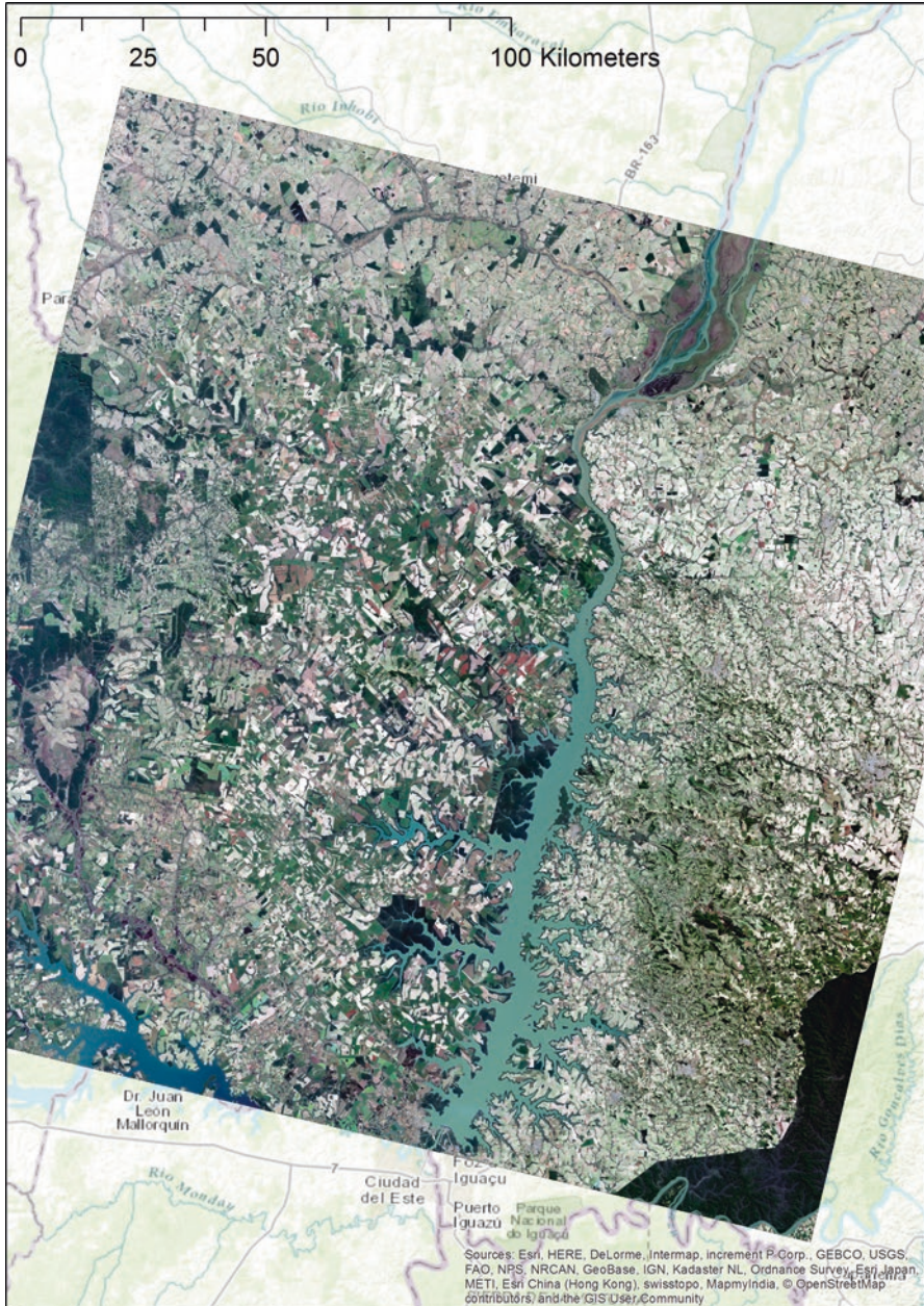
Fig. 5.21 The satellite image of Itaipu Dam on the border between Brazil and Paraguay (surface area 1350 km 2 , max. Length 170 km, max. Width 12 km) captured from Landsat 8 (August 11, 2016)
