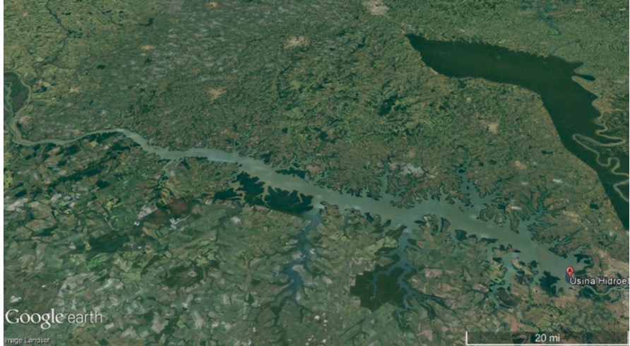
Fig. 5.16 Itaipu Dam: Brazil-Paraguay, 25^{\circ}24'31''\text{S} 54^{\circ}35'21''\text{W} , capacity: 14,000 MW (creates Itaipu Reservoir, total capacity 29 \text{ km}^3 , catchment area 1350,000 \text{ km}^2 , surface area 1350 \text{ km}^2 , max. length 170 \text{ km} , max. width 12 \text{ km} ). Source: Google Earth, 2016
