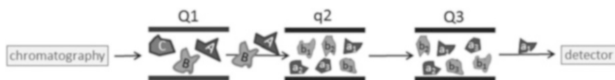
Fig. 1 Theoretical background of HPLC-coupled tandem mass spectrometry (HPLC-MS/MS). After chromatographic separation structurally similar molecules (“A,” “B,” and “C,” with “A” being the desired analyte) may coelute from the HPLC column and are ionized in the source of the mass spectrometer at the same time. These compounds enter the first quadrupole (Q1) where ions are selected regarding their m/z -values. And only those ions with a distinct m/z -value are able to pass this quadrupole. But some compounds (e.g., “A” and “B”) may have very similar m/z -values and therefore, cannot be discriminated. Both ions enter the collision cell (q2) and will be fragmented (“ a_1 – a_3 ” and “ b_1 – b_3 ”). To discriminate between molecule A and B a specific fragment of A (e.g., fragment a_1 ) is selected in the third quadrupole (Q3) and finally passes through to the detector. Other precursor or fragment ions can be selected by changing quadrupole parameters, which allows a simultaneous detection of numerous analytes in one analytical run
