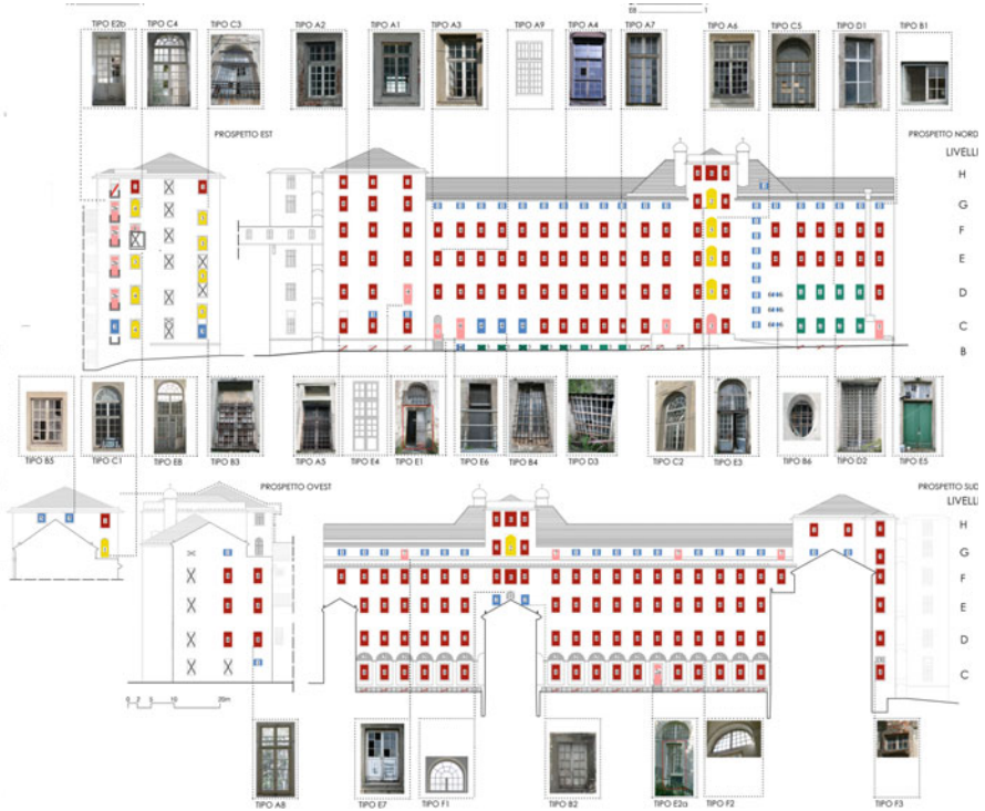
Fig. 7.9 Abacus of the northern wing windows (Borea, S., Brustio, M., Cafferata, D., Geromino, V., Moggia, C., Segantin, F., Szentirmai, B. 2012. Post-graduate School in Architectural Heritage and Landscape, University of Genoa)
