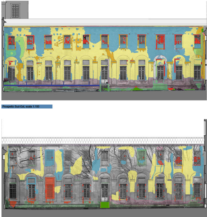
Fig. 1.2 Data acquisition and processing. Conservation status of the façades of the western wing (Biasio, M., Del Monte, M., Galesio, P., Kyuyeon, K., Migogna, T., Pedroni, M., Pescetto, M. Roccon, B. 2014. Post-graduate School in Architectural Heritage and Landscape, University of Genoa)
