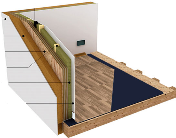
Fig. 8.5 Detail of new insulated internal layers for the university accommodations (Bresolin, G., Stagnaro, I., Tomasetti, G. (2012). Master course in Architecture)
