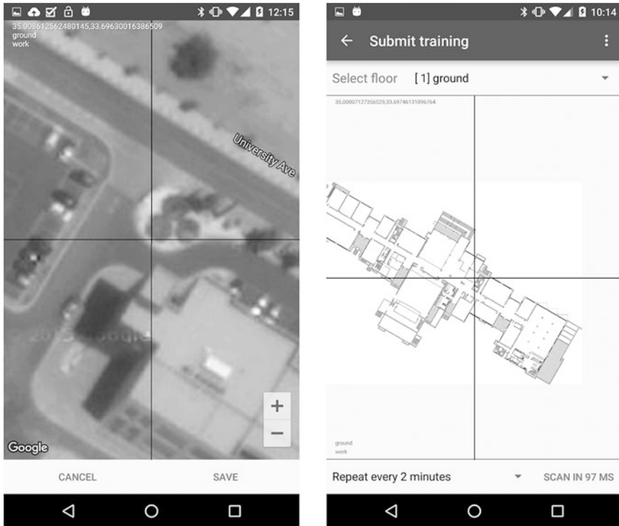
Fig. 2 Aligning the blueprint with the real world using satellite imagery ( left ). In the training phase, the users select their exact position—at the correct floor—and then start a new scan. Optionally, the user can select an automatically triggered scan that repeats periodically ( right )
