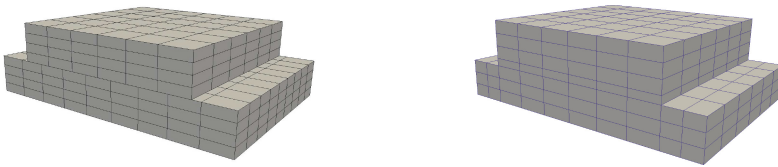
Fig. 10. Finite element mesh of the contact case (left) and of the continuum case with one layer of elements between the two bodies (right)
