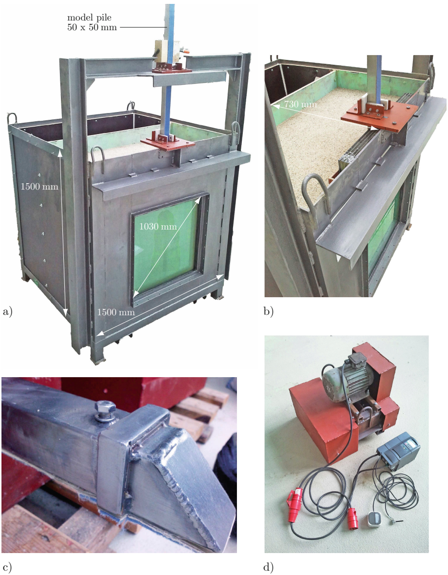
Fig. 8. Experimental investigation of vibro-injection pile installation. (a) Filled test chamber with glass panel and model pile. (b) Detailed view of the glass panel, pile guide, and model pile. (c) Tapered pile toe with welded-on collar and bolt closing the injection tube. (d) Self-made vibrator with controller (frequency converter). Reprint from [141, p. 117] with permission of Springer.
