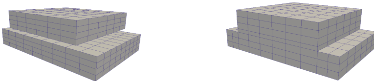
Fig. 15. Finite element mesh of the contact case (left) and of the continuum case with one layer of elements between the two contact bodies (right)
