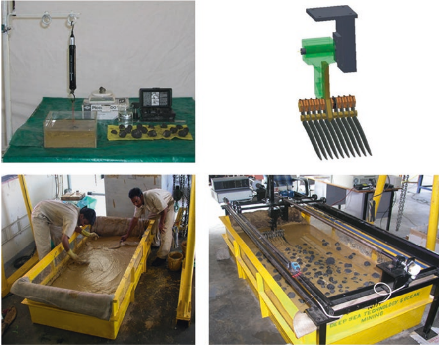
Fig. 10.9 Experimental studies on pickup devices for manganese nodule mining
