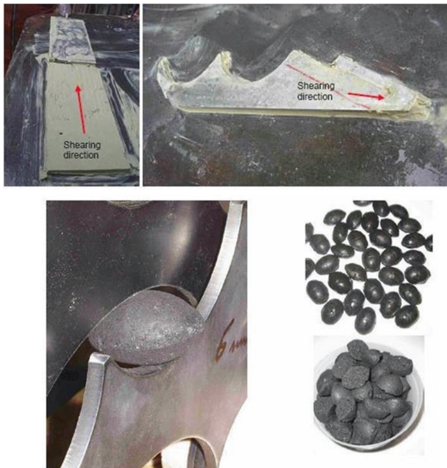
Fig. 10.10 Experimental studies to determine forces for breaking nodules
