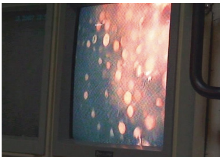
Fig. 10.23 Laying of artificial nodules being dropped from vane feeder
