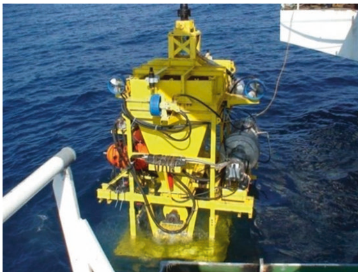
Fig. 10.25 Artificial nodule laying system being launched
