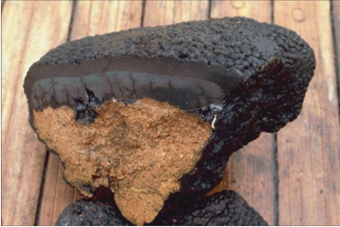
Fig. 3.1 Cobalt-rich manganese crust covering a hyaloclastic substrate rock; thickness of the crust about 8 cm; sample from a seamount slope in the Central Pacific Basin. The fracture surface shows a younger upper and an older lower layer. The latter is strongly impregnated by carbonate-flourapatite
