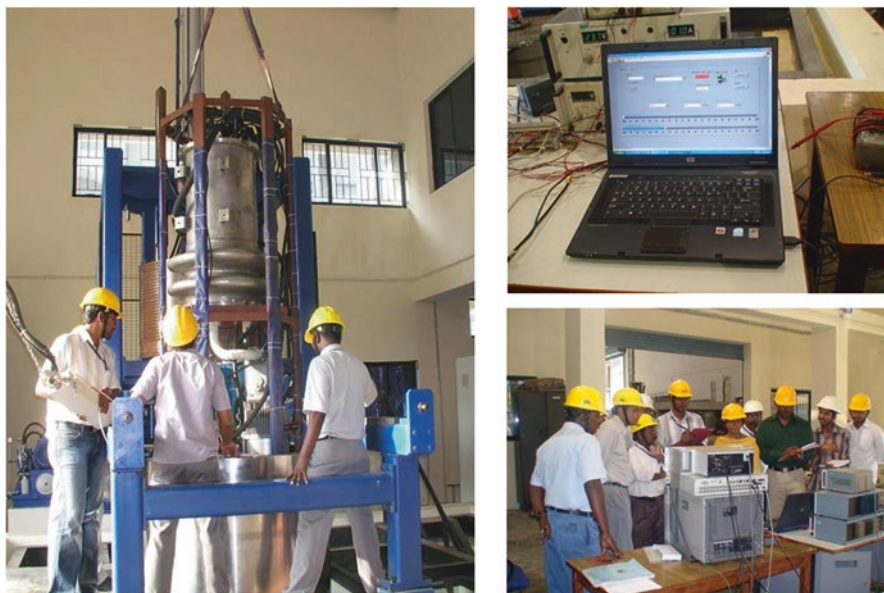
Fig. 10.6 Testing of underwater hydraulic systems in hyperbaric chamber
