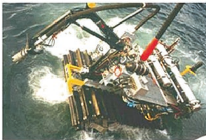
Underwater Mining System with manipulator and cutter for 500 m depth
