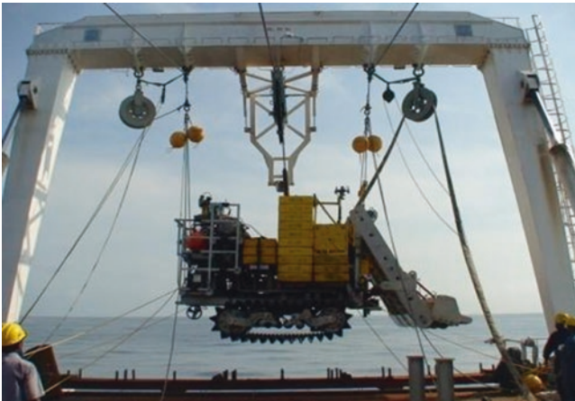
Fig. 10.37 Launching of underwater mining machine
