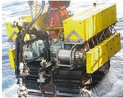
Enhanced Underwater Mining System for 500 m depth
