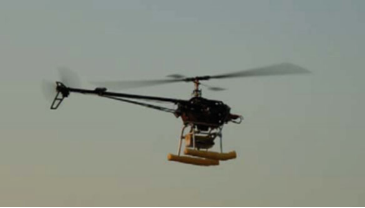
Fig. 8.2 THeli260 unmanned helicopter
