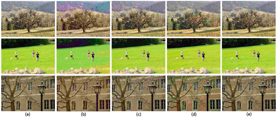
Fig. 1. (a) Original image, compression results using (b) Standard JPEG scheme (c) Defocus cue based scheme at quality parameter 3, compression results using (d) Standard JPEG scheme (e) Defocus cue based scheme at quality parameter 5.
