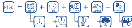
Fig. 3. Here, the individual specific exposure ( ISE ) is accomplished with particular process knowledge to allow decision making and situational prediction in form of a predictive individual specific exposure ( PISE ).
