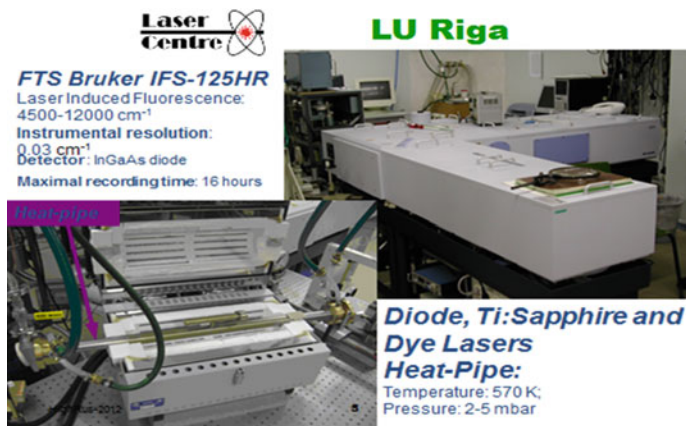
Fig. 16.2 The experimental setup that is exploited in the Laser Center of University of Latvia and Institut für Quantenoptik, Gottfried Wilhelm Leibniz Universität Hannover with outstanding laser facilities combined with very high-resolution Fourier spectrometers. The setup enables one to record LIF spectra with instrumental resolution comparable to Doppler width in the visual and infrared region of spectra [2]
