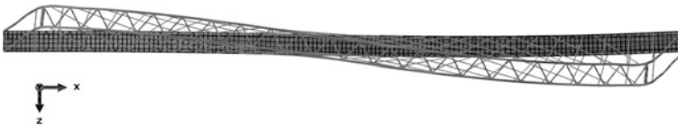
Fig. 6 Second estimated buckling mode
