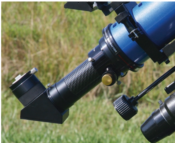
Fig. 5.5 The dual speed focuser on the author's 102 mm refractor (James Chen)
