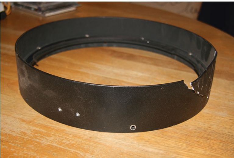
Fig. 3 Another angle of the cracked Schmidt corrector plate cell
