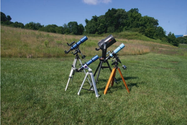
Fig. A16 The author’s telescopes featuring an Alt-Az with slow motion controls, two German equatorials, and computerized GoTo Mount (James Chen)
