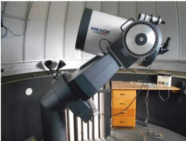
Fig. 5.3 Meade LX-200 16-in. SCT installed in a dome (Hands-on-Optics archive)
