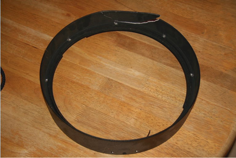
Fig. 2 The cracked Schmidt corrector plate cell
