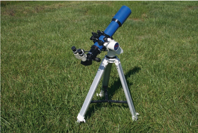
Fig. A17 Alt-Azimuth mount with slow motion controls (James Chen)
