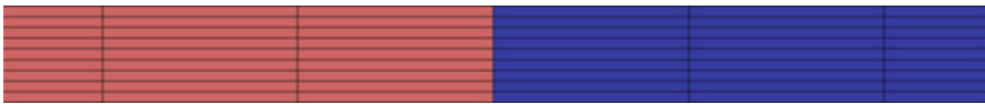
Fig. 4 Detail of the interface between two subdomains for narrowing along the y -coordinate in 3D for graph ( left ) and geometric ( right ) partitioner
