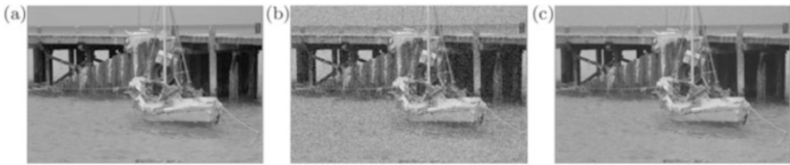
Fig. 2 (a) Original clean image of size 2048 \times 3072 , (b) Noisy image with Gaussian noise with zero mean and 0.03 variance (PSNR=15.66), (c) Denoised image with weight \lambda = 7 in (2)
