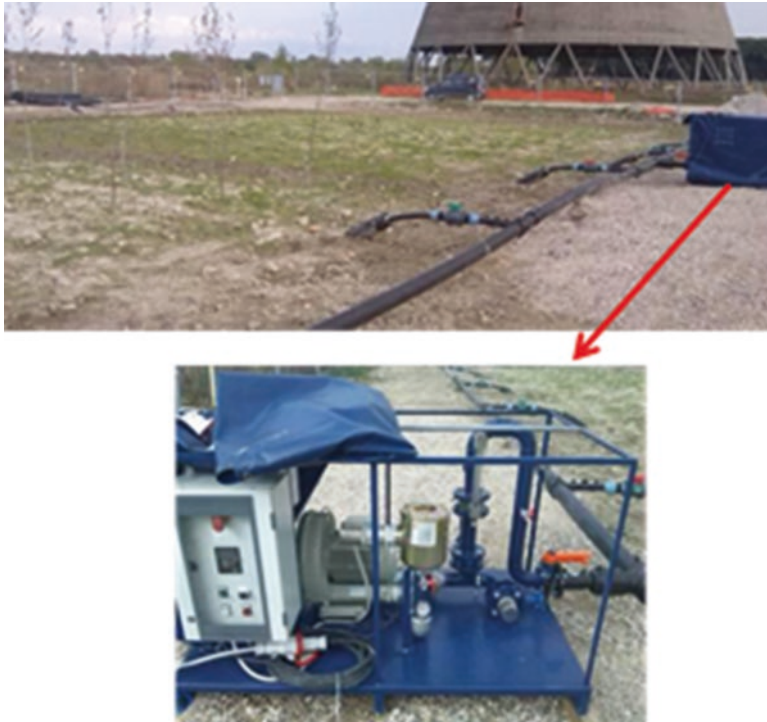
Fig. 3.11 Structure of biosparging system into pilot field
