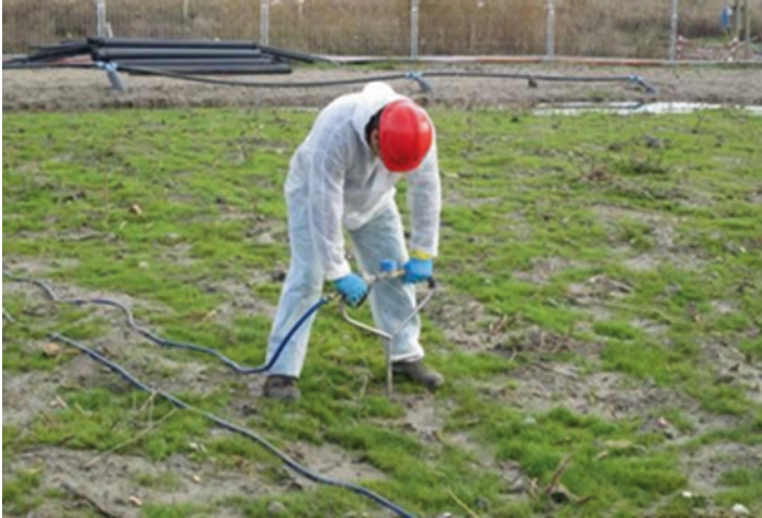
Fig. 3.9 Direct inject into field with injector pole
