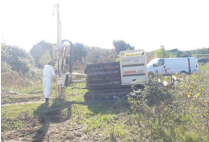
Fig. 3.1 Core drill used to collect soil
