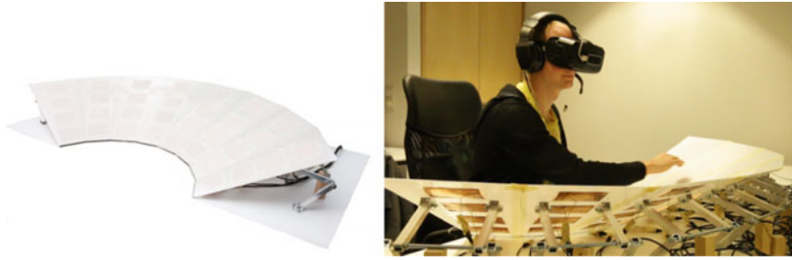
Fig. 6 Left Curved device implementing free-form capacitive sensor surfaces— Right Natural curvature supports interaction in Virtual Reality scenarios
