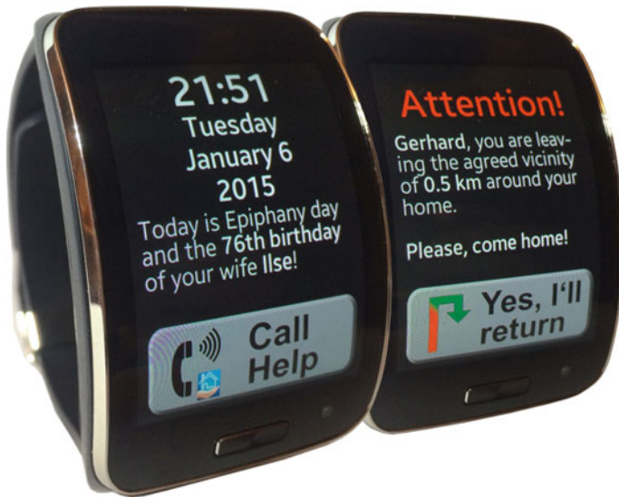
Fig. 5 Smartwatch Samsung Gear™ S with assistance app displaying communication and orientation information (holidays, birthdays, ...) on the left and an advice to return to home after leaving an agreed area (geofencing) on the right
