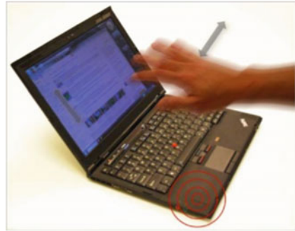
(b) Gestures Recognition using ultrasound measurement on laptop. The depicted figure is taken from [10]
