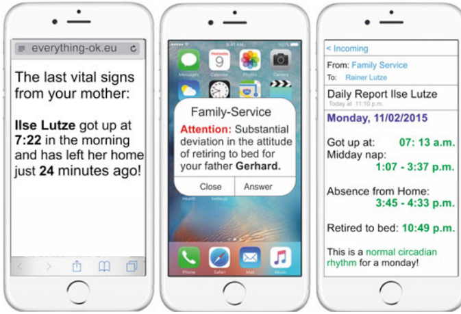
Fig. 6 Services for family members delivered by the LTAS: on demand requests for the last vital signs from the person in need of support/care ( left ), warning of substantial deviations of the used circadian cycle ( middle ), regular reports summarizing the last day ( right )
