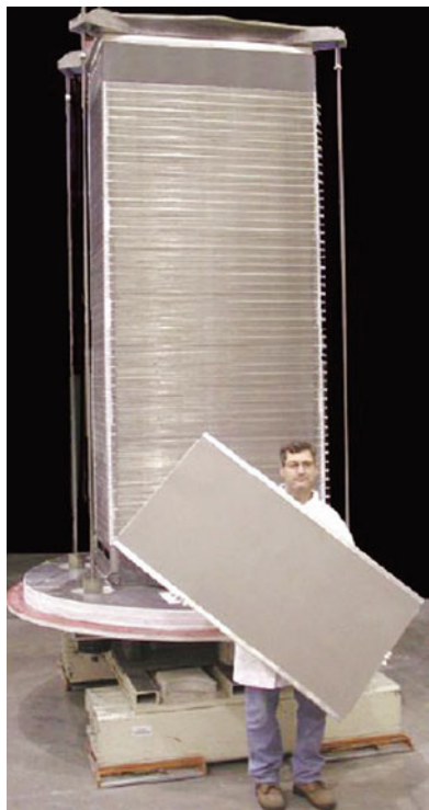
Fig. 19 Full size molten carbonate fuel cell and stack. Reprinted from [362], with permission of John Wiley and Sons
