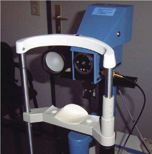
Fig. 7.6 Chromatic pupillography equipment in our laboratory. The stimulus is provided by a mini-Ganzfeld color LED stimulator to one eye and the consensual pupil light reflex of the nonstimulated fellow eye is measured by the compact integrated pupillograph (AMTech GmbH, Dossenheim, Germany)
