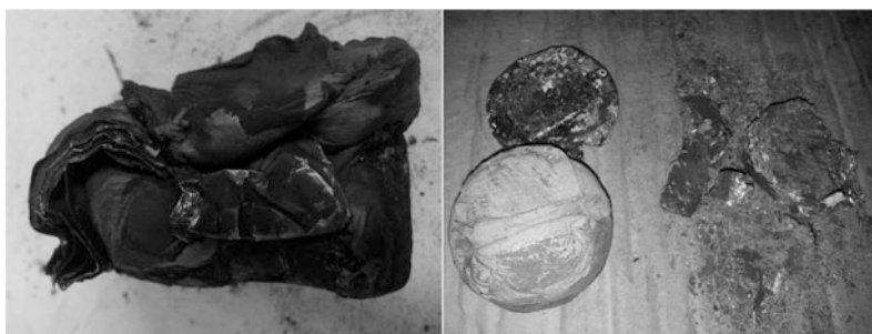
Fig. 4 Sample of battery after preheating in air at 500 °C and then co-melting with pure aluminium
