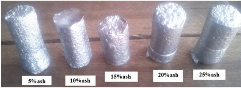
Plate 2 Surface appearance of aluminum ingots casted from the blended sand
