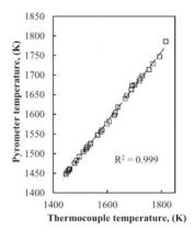
**Fig. 5** Pyrometer calibration using levitated copper droplets of different mass
