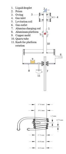
Fig. 3 Schematic diagram of levitation coil
