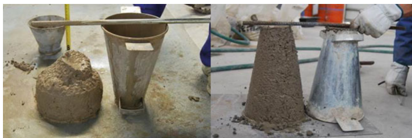
Fig. 2 Abrams cone of the mixture P-concrete with natural aggregates and the mixture EM1-concrete with EAFS and fibers
