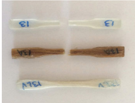
Fig. 7 Tensile ruptured specimens for each volume fraction of curaua fiber incorporated into the epoxy matrix
