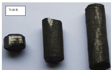
Fig. 7 Photograph of samples obtained in optimal technological regimes: bulk TiAlB rods before mechanical treatment
