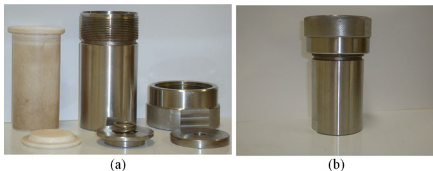
Fig. 3.5 Hydro-/solvothermal synthesis reactor. (a) Teflon-lined stainless steel cap; (b) closed reactor
