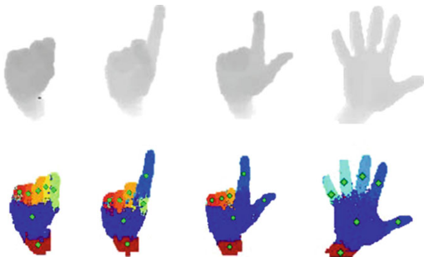
Fig. 7.8 A set of representative results of the recognized hand parts via the trained RFs on real data
