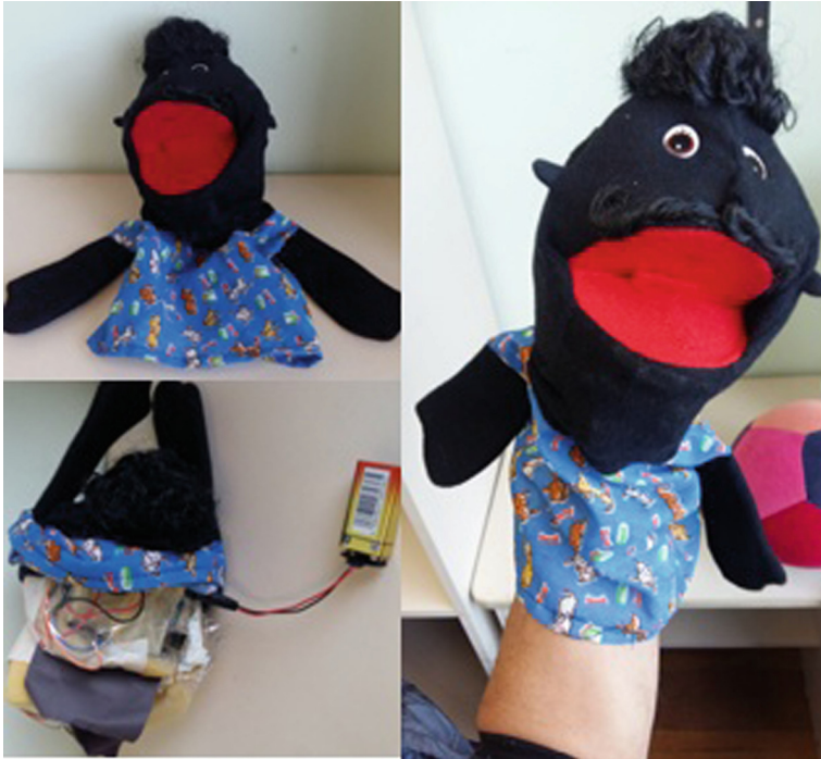
Fig. 15. Puppet Module with Arduino Micro, Bluetooth, RFID receptor (inside the nose) and power battery.
