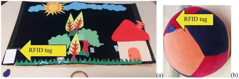
Fig. 16. Ball with RFID tag (real object) comes close to a scenario (abstract object) also with RFID tag.
