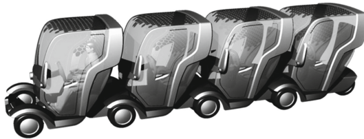
Fig. 4. ESPRIT stackable electric vehicles.
