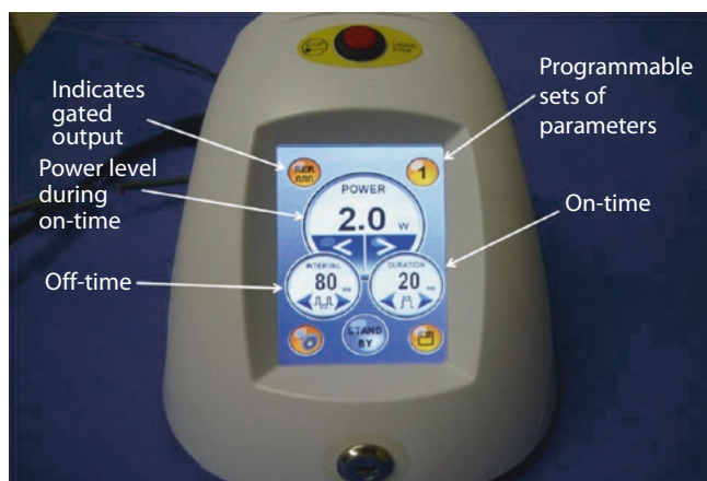
■ Fig. 4.5 This 810 nm diode laser has a limited number of variables that may be controlled directly
