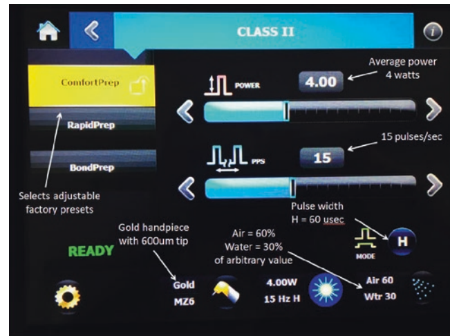
■ Fig. 4.6 This 2780 nm Er,Cr:YSGG laser has a choice of two pulse widths. It allows control of average power but energy per pulse and peak power must be calculated. Levels of auxiliary air and water are set as percentage of arbitrary values determined by supply to the individual dental suite
