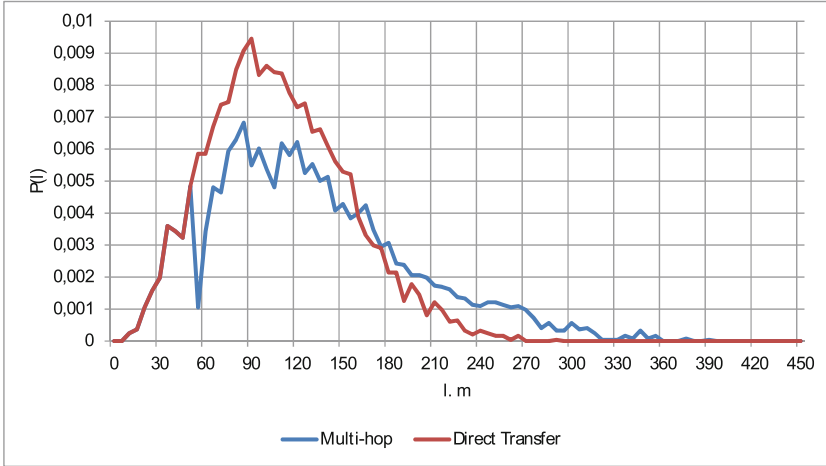
Fig. 5. Comparison of the average direct transfer distance and average multi-hop distance for the swarm of nodes within the cylinder
