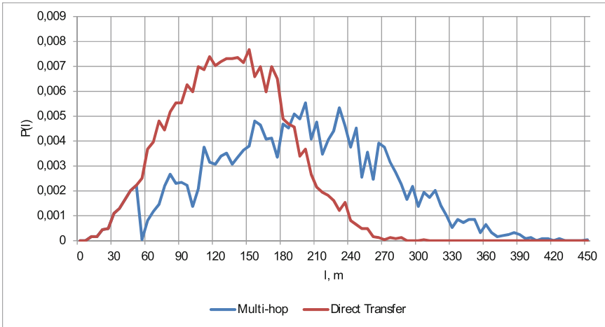
Fig. 6. Comparison of the average direct transfer distance and average multi-hop distance for the cubic swarm of nodes
