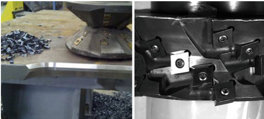
Fig. 1 On the left , an example of a milling head tool. On the right , the milling head tool model employed in this project
