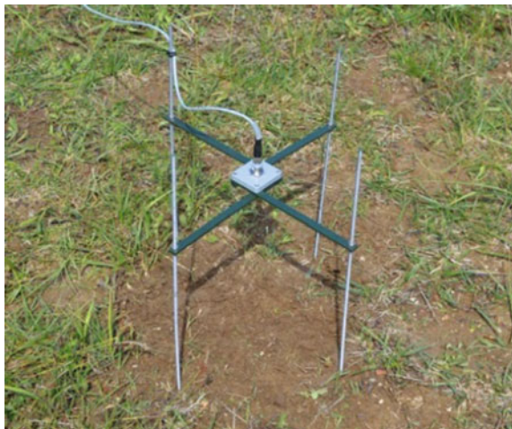
Fig. 3 The UB800 ultrasonic sensor was selected and used
