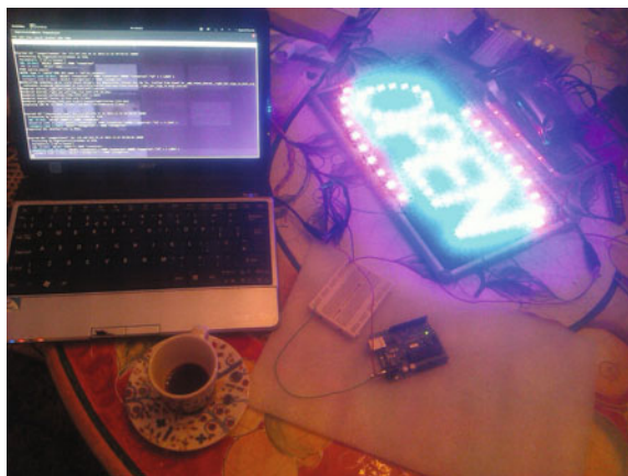
Fig. 4.16 ( Left ) Internet-enabled open sign under development (photograph Rory Gianni); ( right ) electric imp module (photograph http://www.electricimp.com media resources)
