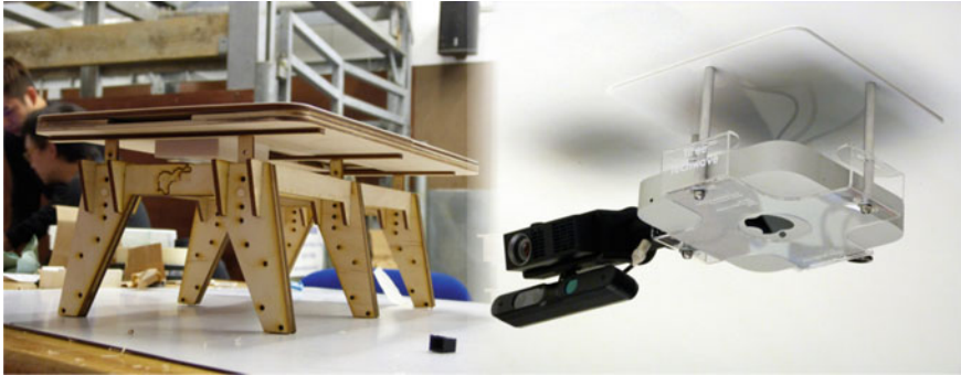
Fig. 4.19 Custom table design ( left ) and ceiling enclosure for projector and depth camera ( right )
