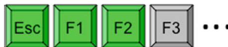
Fig. 9.2 Layout matters (from Dix et al. 2004). The key sequence F1–F2 meant “exit and save if modified”, whereas F1–esc–F2 meant “exit without saving”. This was fine on keyboards where the function and escape keys were separated, but on the above layout led to accidentally pressing the escape when trying to hit F1–F2
