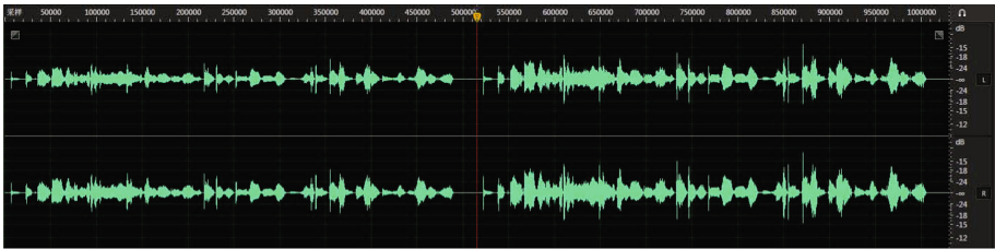
Fig. 2. The figure on the left of the red line shows the wave form of the original signal, and the one on the right is a example of DVF-ISM processed audio when sound source is located 30 cm away from listeners. (Color figure online)
