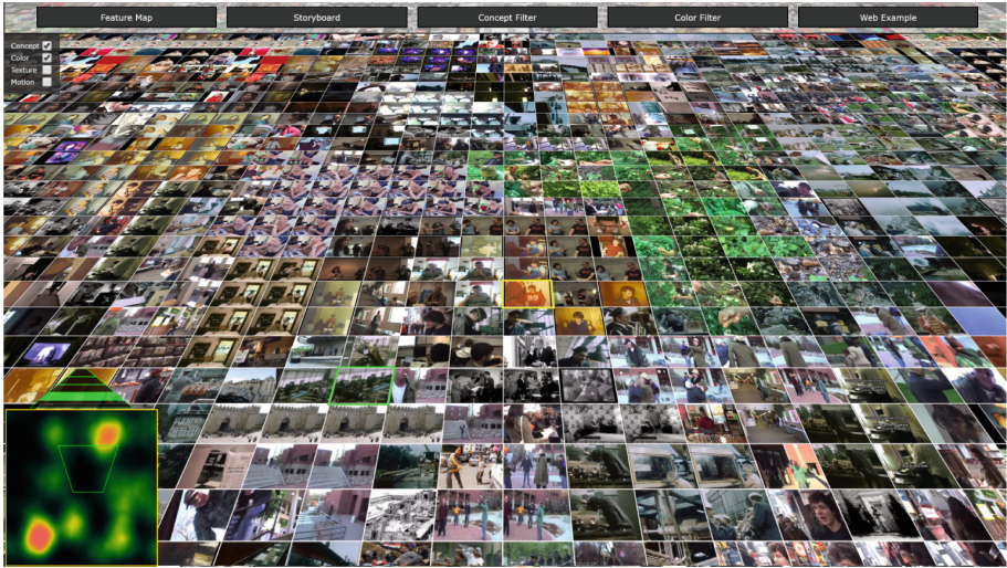
Fig. 1. Feature Map: the main view of our interface arranges keyframes according to a similarity criteria, which can be selected on the left. The current hierarchical layer is visualized by a pyramidal indicator at the bottom left. The minimap below indicates the currently visible section and includes a heatmap that summarizes the current search activity of all users. Filter Views can be selected via a navigation menu at the top. (Color figure online)
