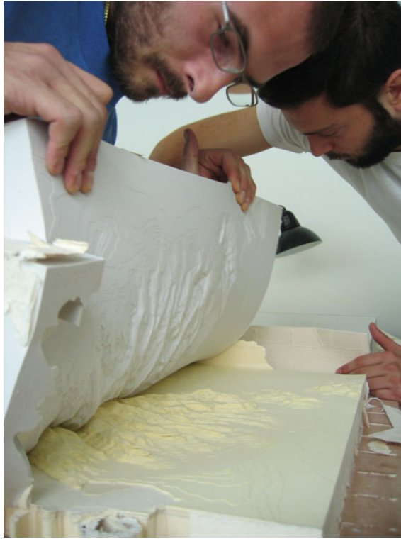
Fig. 8.4 Cardboard positive and silionic rubber mold
