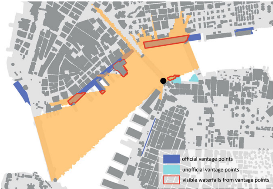
Fig. 5.7 “Where from can I watch the NYC waterfalls?” The computation of simple 2-D isovists was enough to assess the vantage points on the waterfront of The New York City Waterfalls project by Olafur Eliasson in 2008. The City of New York wanted to grasp the number of people visiting the installations diffused over several locations. By catching people at these vantage points it was possible to concentrate advertisement and initiatives (credits Study and image by the author, Senseable City Lab, MIT)
