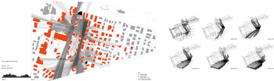
Fig. 7.4 Isovists from paths: 2D isovist along a path in an urban environment and 3D isovist along a path in the 9/11 Memorial Museum [SUPERSPACE @ Woods Bagot & Computational Design Research group (CDR) @ Aedas]
