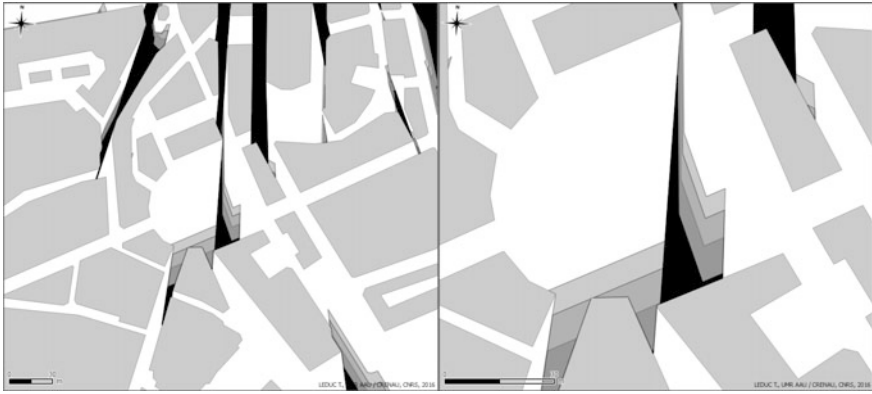
Fig. 6.4 The four set of v-lines with a zoom in on the Royale square (right). The black (resp. dark-grey, grey, and light-grey) polygons correspond to portions of ground space in which the punctual generator located at 42 m (resp. 32, 22, and 12 m) from top of the Bretagne tower is visible
