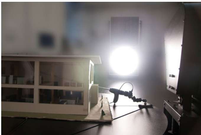
Fig. 10.4 Simulation of a sky in Betanit virtual dome artificial sky ( credits The author)
