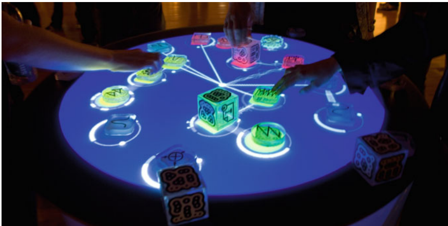
Fig. 15.3 The ReactTable an electronic musical instrument example of tangible user interface, by Daniel Williams from NYC, USA https://www.flickr.com/photos/84466661@N00/539568298/ (creative commons)
