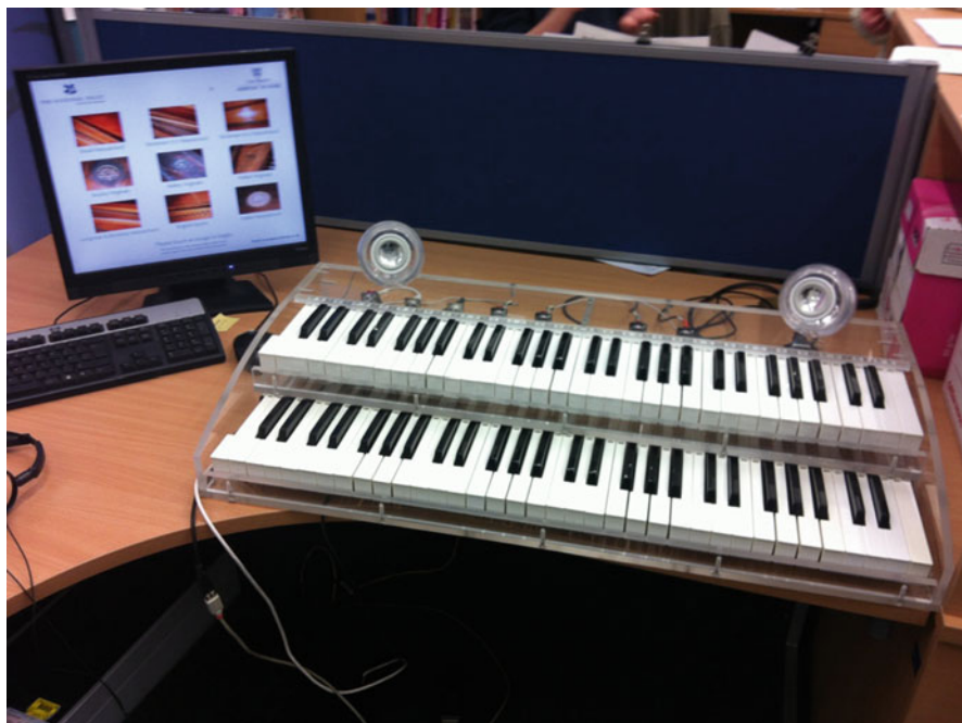
Fig. 4.2 The two-manual MIDI interface for the digital harpsichord
