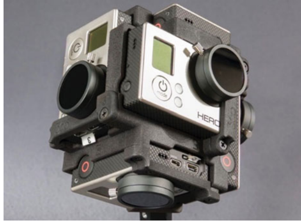
Fig. 8.2 Six GoPro cameras in freedom 360 setup (Go Pro 2014)
