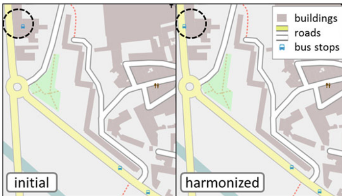
Fig. 1.9 One bus stop is far from the road and harmonized by displacement
