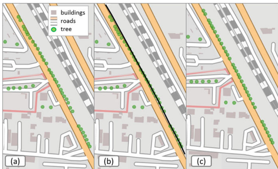
Fig. 1.6 (a) Inaccurate trees overlapping a road. (b) computation of an offset on the side of the road with trees. (c) trees aligned on the offset line
