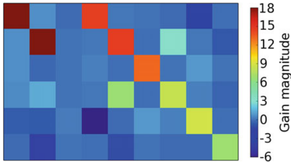
Fig. 5 A visualization of a gain matrix as it is computed from LQR on the momentum equations. It is interesting to see that off-diagonal terms, which are not obvious to design by hand, contribute significantly to the feedback. For instance we can see that the lower left part of the matrix exploits coupling between linear and angular momentum and uses angular momentum in order to correct errors in CoM and linear momentum tracking (Figure taken from Herzog et al. [13])
