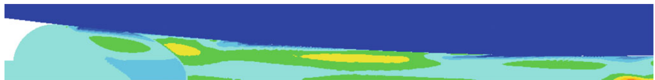
Fig. 8 Concentration of silicon in wt% from 0.75 to 1.05 in step 0.03 wt%. Blue areas are depleted in Si. The mushy zone is visible to the left. The shrinkage flow causes the mixture concentration to appear depleted down to the fully solid
