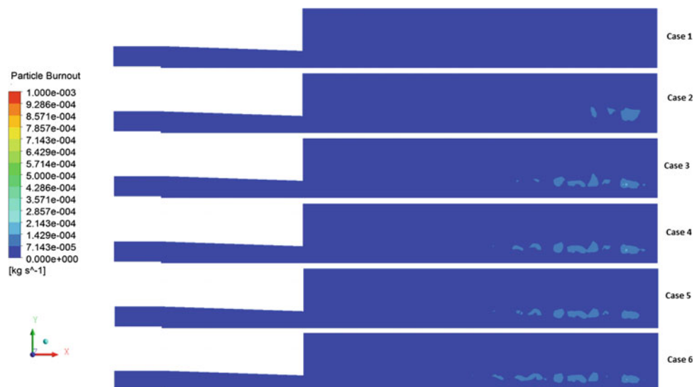
Fig. 6 Variation of 'SPL washed' particle burnout at different conditions in a simulated 2D tuyere region
