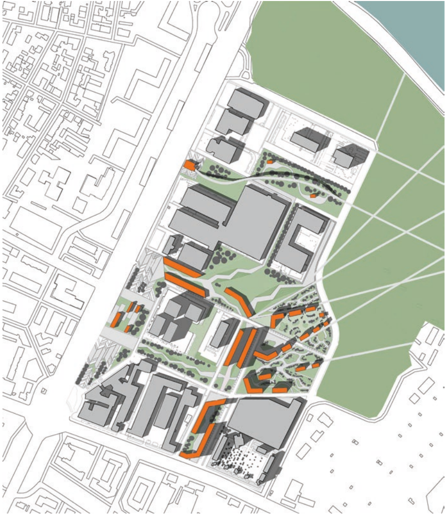
Fig. 3.15a Permeable strategy to integrate industrial and commercial buildings with new housing and services. Discover the nature. (Source: International Workshop Design along the river. Turin, September–December 2014. Politecnico di Torino. Tutors: Ingaramo R., Voghera A., Claps P., Mutani G., Mazzotta A. Students: Allevato J., Battafarano I., Sandolo G)
