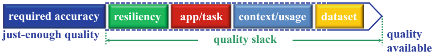
Fig. 1.20 Slack between the quality available from the processing platform and the actual quality required by the specific chip, application, usage scenario and dataset
