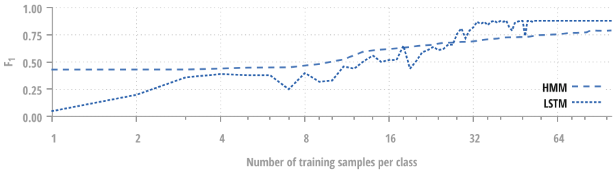
Fig. 4. Early learning behavior, averaged over 10 random folds. HMMs outperform the LSTM network where very little training data is available, while the latter performs better with more than 28 training sequences. Note that the x-axis is scaled logarithmically.
