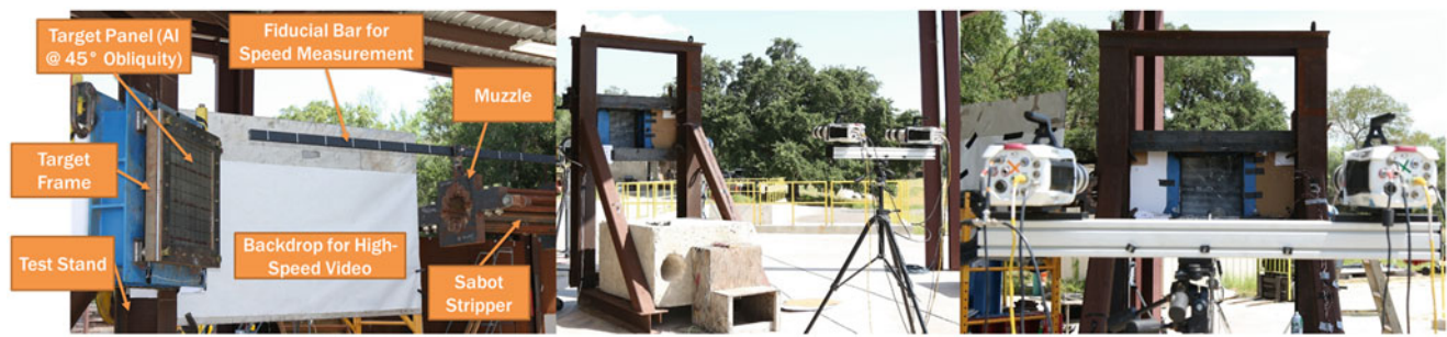
Fig. 63.4 Typical DIC setup for a bird-strike test: in this case the target is a flat aluminum plate
