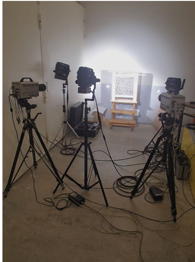
Fig. 4.1 Stereo-correlation device comprising high speed camera and large scale target with coarse speckle pattern
