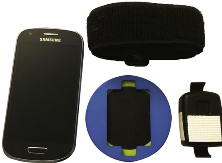
Fig. 6 Components of the SIRRACT sensor kit supplied to subjects is shown. At lower left is the system smartphone. At upper center is the ankle worn Velcro attachment for the sensor. The wireless charging unit with a recess accepting the sensor is at lower center. The motion sensor system is shown at lower right
