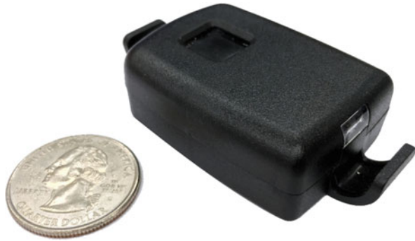
Fig. 3 Inertial sensor system within a sealed enclosure
