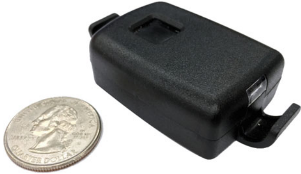
Fig. 3 Inertial sensor system within a sealed enclosure
