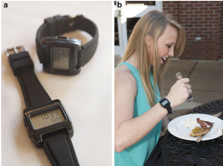
Fig. 1 The commercially available Bite Counter, now marketed as the ELMM (eat less, move more) watch; see: http://www.myeimm.com . (a) Bite Counter close-up. (b) Bite Counter in situ
