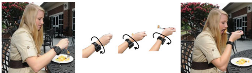
Fig. 2 Wrist roll motion during the taking of a bite of food occurs regardless of the type of food or utensil
