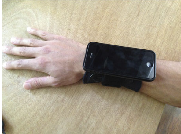
Fig. 5 Audio was captured by a smartphone attached to the wrist running an off-the-shelf audio recording mobile application
