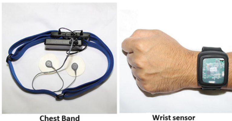
Fig. 7 AutoSense chestband and inertial wristband sensors used in user studies. Wrist sensors were used only in Study 2 (with newly abstinent smokers)
