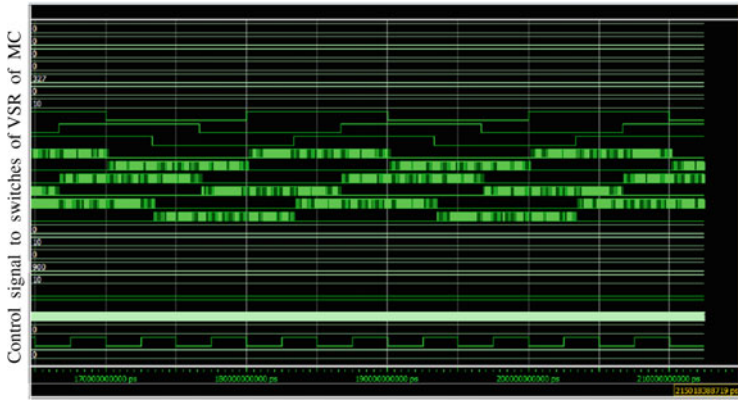
(a) Control signal to VSR of MC
