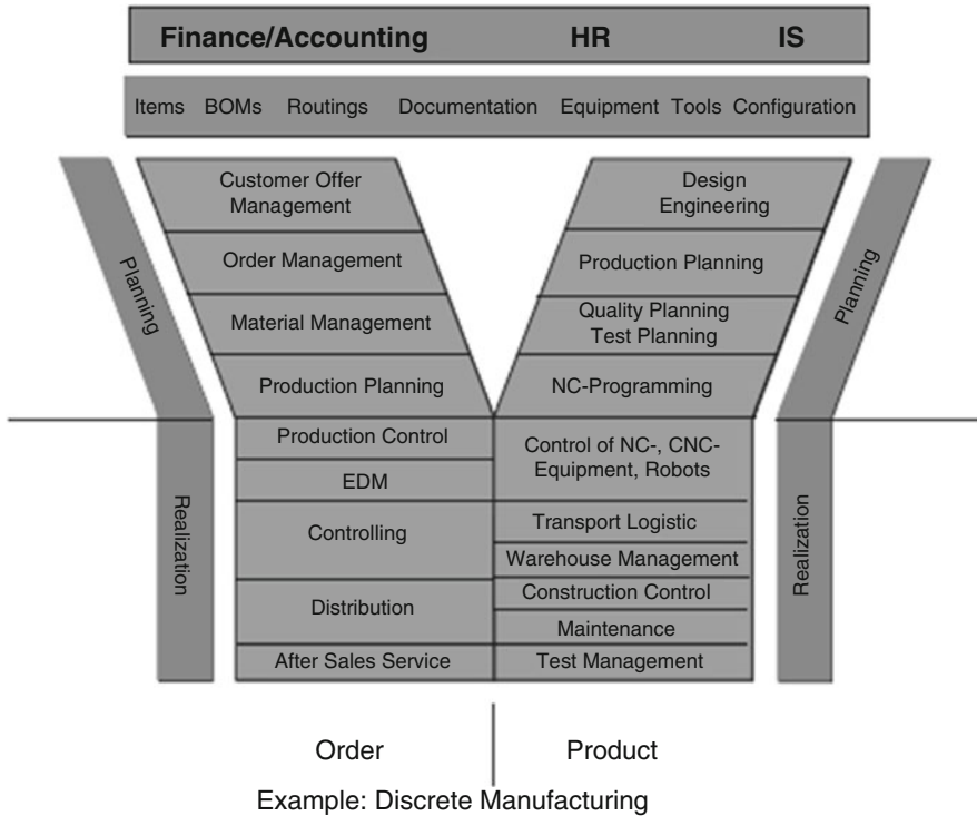
Fig. 6.8 “Y-model”: reference model for industrial enterprises (after A.-W. Scheer)
