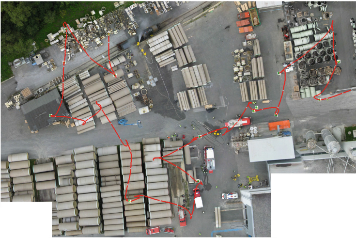
Fig. 5. Part of the overview image stitched from approx. 40 pictures taken during the firefighter's practice along with the UAV's trajectory (red path). (Color figure online)
