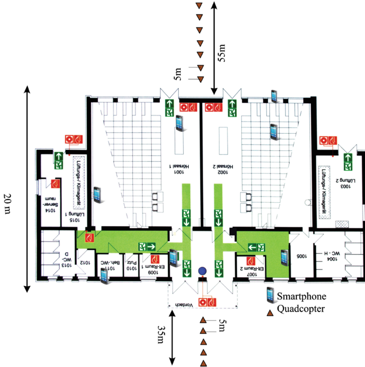
Fig. 2. Floor plan of Leonardo da Vinci building at technical university of Ilmenau. Mobile phones were located inside the building. MAV was placed outside the building in front and rear. Positions are marked accordingly.
