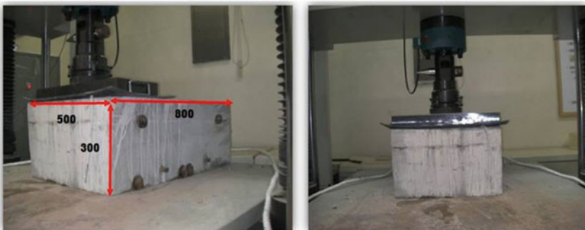
Fig. 23.4 Compressive strength Load Test
