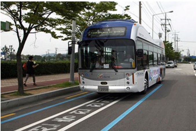
Fig. 2.4 OLEV bus in Gumi. The blue lines indicate the location of the underground power supply cables
