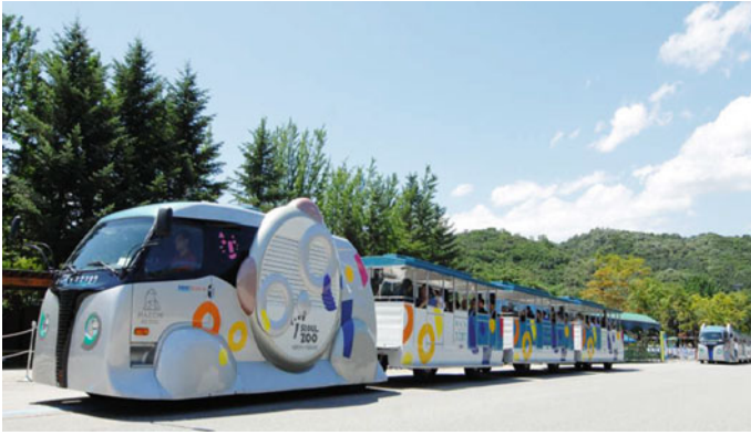
Fig. 2.3 OLEV tram installed in Seoul's Grand Park
