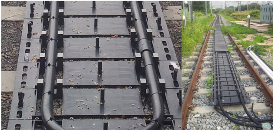
Fig. 17.8 Photographs of developed 128-m transmitter track
