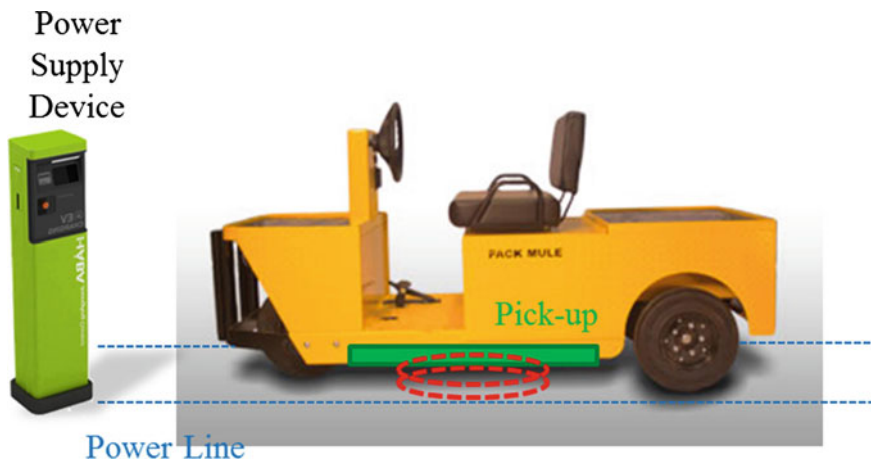
Fig. 18.2 Concept of wireless power transfer electric carrier for airport application (source drawing)
