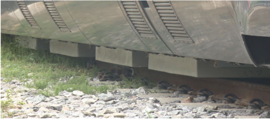
Fig. 17.11 Photograph of installed four pickup units
