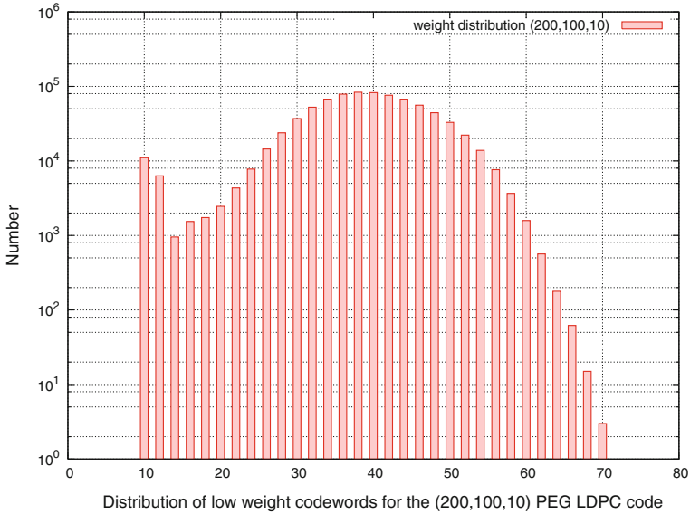
Fig. 14.17 Distribution of codeword weights responsible for non-MDS performance, for the (200, 100, 10) PEG LDPC code
