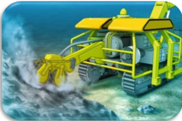
Fig. 1. Rock grinding of the underwater construction robot [4]
